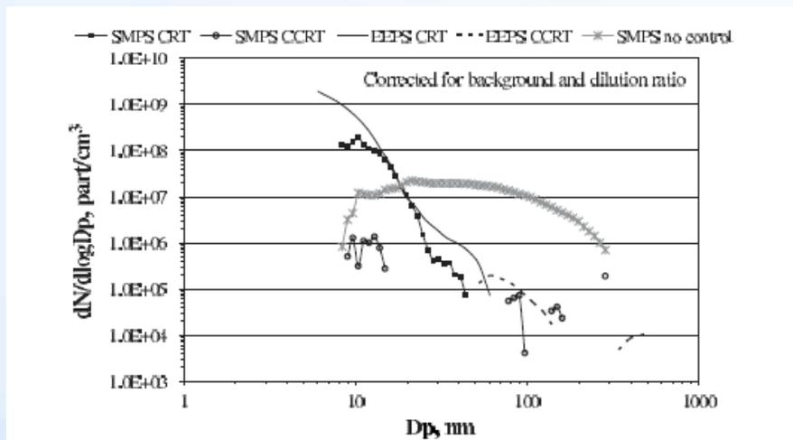
Fig. 5. SMPS and EEPS size distributions for the CRT, CCRT, and uncontrolled case.
