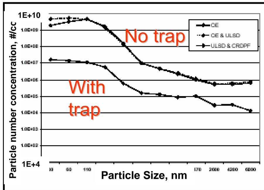
Figure 8: ELPI Particle size distribution over the CBD cycle during phase II emissions tests
