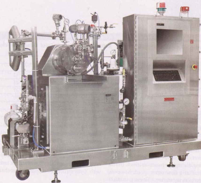
The system was developed to achieve very narrow submicron particle size distributions through high-energy, high-flow, multiple-pass grinding.
